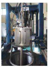
Pressure testing of Subsea Transformer
