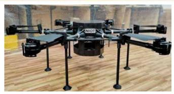
Heavy Lift - Hexacopter Drone capable of lifting 10kg instrumentation payload
