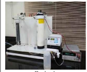
Flow bench Precipitation sensor calibration
