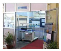
Ocean Observation system is developing Indian Tsunami Bottom Pressure Recorder (ITBPR). The Tsunameter Test Facility was established in NIOT to test the functionality of ITBPR by simulating tidal variations. The imported BPR measured the sea level variations from the seabed. The mean value (i.e depth) removed, the sea level variation is feed to vertical arm which is fixed with the pressure sensor to test the functionality of ITBPR.
