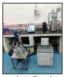
In-situ Thermal conductivity measurement reactor
