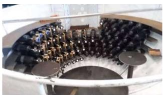
HSSS components and oxygen cylinder arrangements
