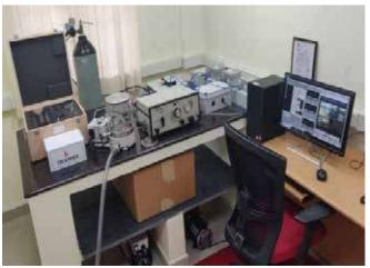
Digital Gas Piston Gauge-Barometric pressure sensor calibration
