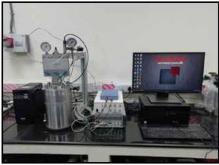
Acoustic wave velocity measurement reactor
