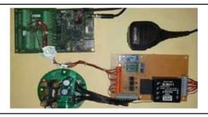
Prototype DSP based stand-alone acoustic telephone unit
