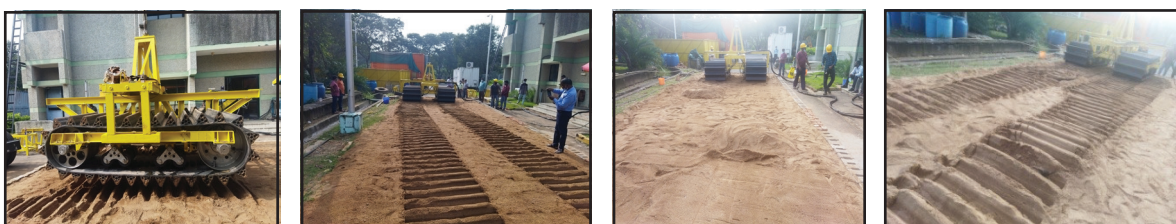
Locomotion test of new driven drum and new HPU on the sand bed
