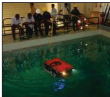
Acoustic Test Facility for calibration of transducers and other system performance tests
