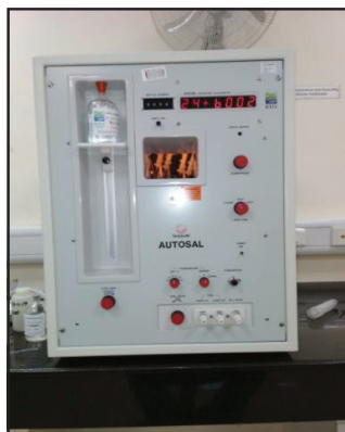
Calibration setup for salinity and precipitation
