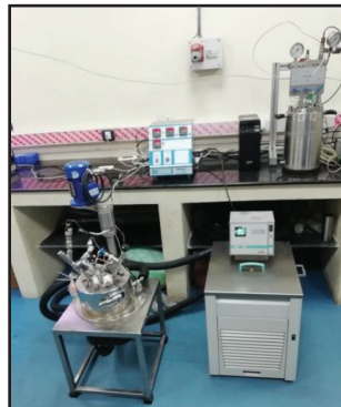
In-situ Thermal conductivity measurement reactor
