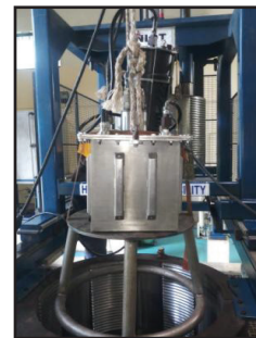
Pressure testing of Subsea Transformer
