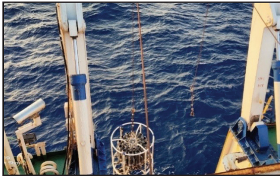
CTD Deployment upto 1000m depth
