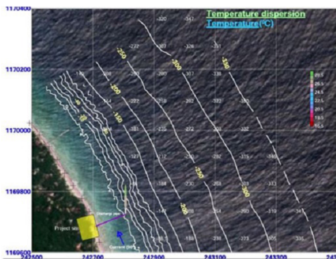
Simulated temperature contours around discharge area
