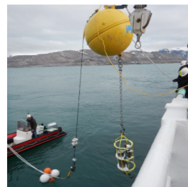
Deployment of IndARC V mooring onboard the vessel MV STALBAS
