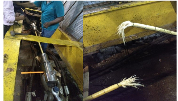
Cable Break load Testing
