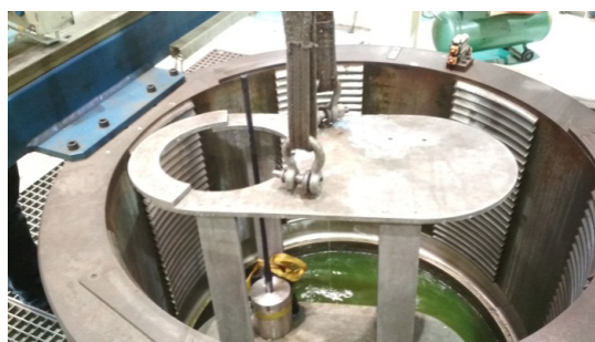
Pressure Test of RF Antenna at Hyperbaric Chamber
