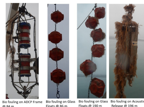
Growth of biofouling on ADCP, Glass floats and Tandem Acoustic release and biofouling on IndArc mooring
