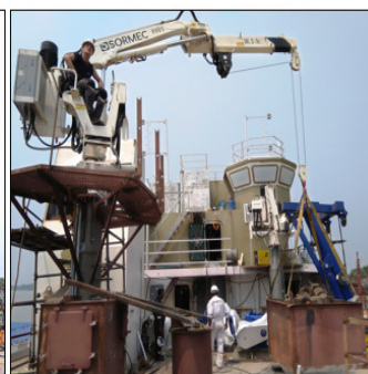
Static and dynamic load test of Deck Crane
