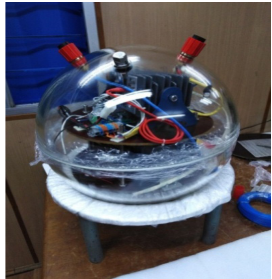
Glass Sphere housing electronics and battery pack
