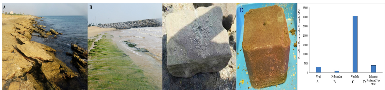
Variation in hardness of stones by compressive strength analysis
