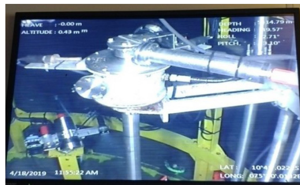
Vane operation at 5418m depth
