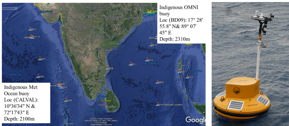
Deployment of Indigenous buoy- PRAKRUTI with I-DAS
