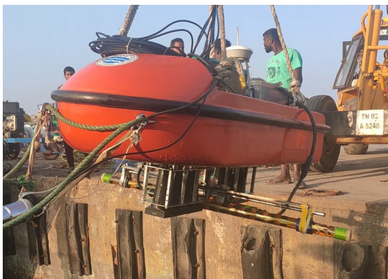
Sea trial with the Mills Cross Array Configuration
