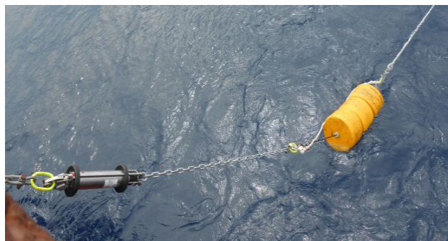
Deployment of Syntactic floats in deep sea mooring
