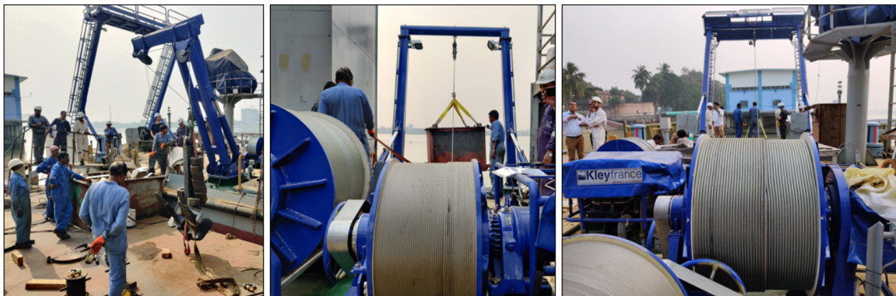
CTD Winch, Oceanographic Winch, General Purpose Winch (Left to right) Load Test of Scientific Winches and Handling System
