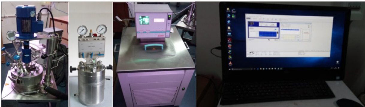
View of Gas Hydrate laboratory set with high pressure and low temperature reactors
