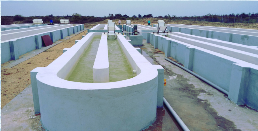
Paddle wheel operated raceway pond
