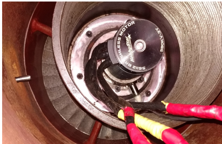
Open Cycle OTEC power module under testing
