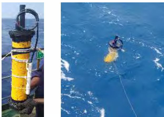
WXBT in lab and during sea trial
