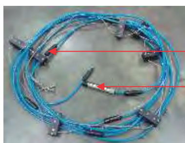
Subsurface temperature measurement string
