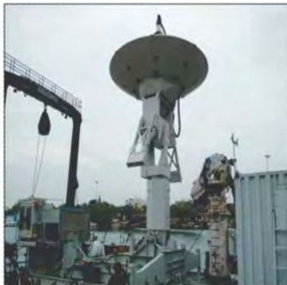
Antenna Fixed onboard for RLV tracking
