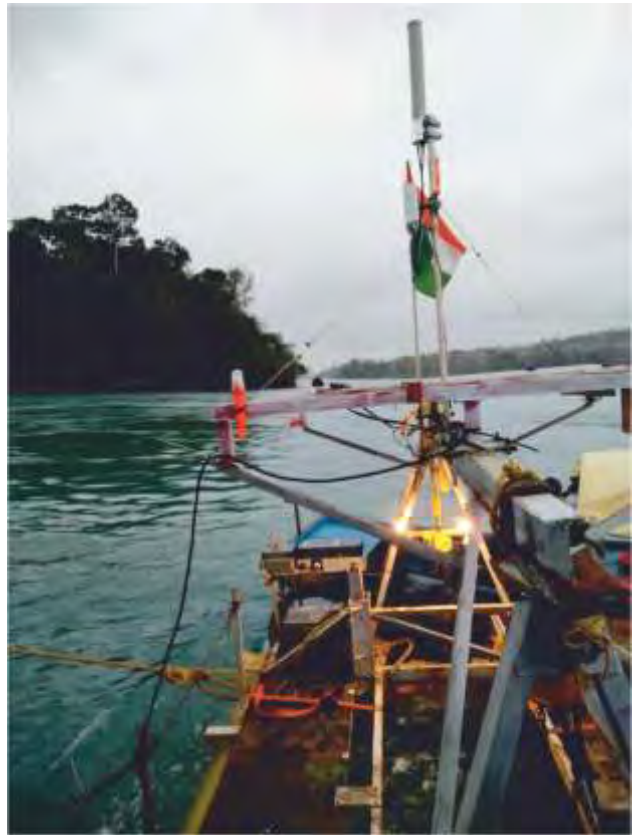
Demonstration of ocean current turbine at Macpherson Strait, Andaman Islands
