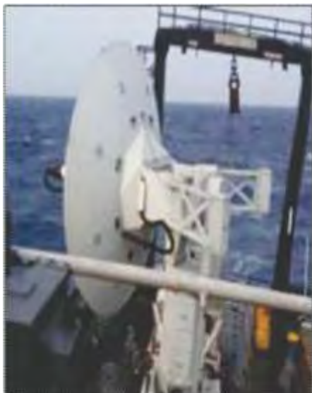
Antenna Fixed onboard for RLV tracking
