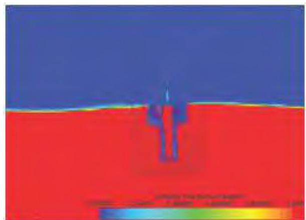
Estimation of water surface and airflow inside the OWC using CFD
