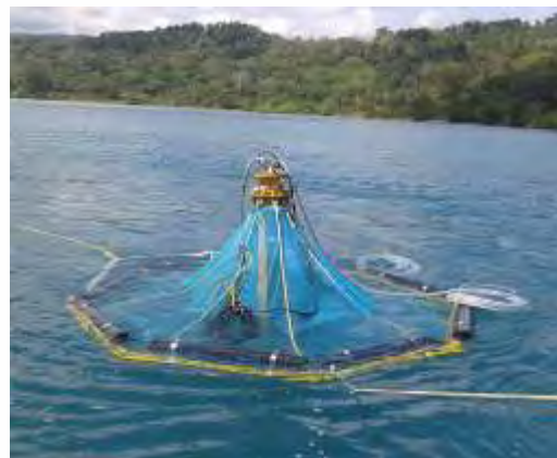
Spar rigid type submerged cage deployed in Andaman
