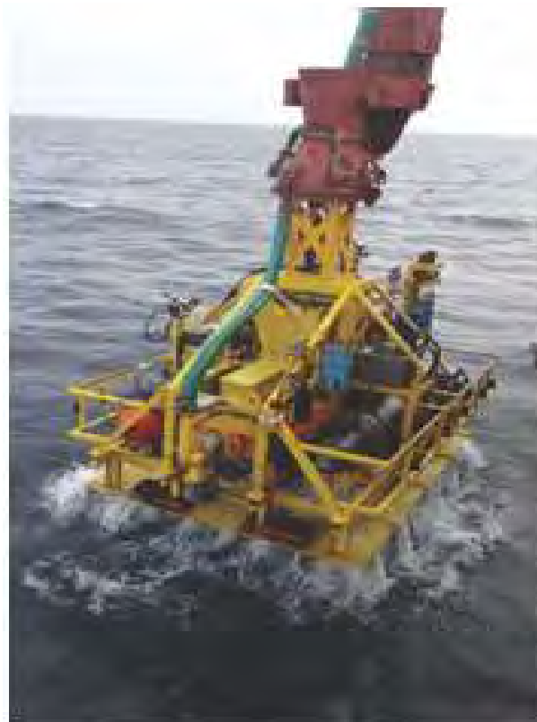
Slurry pumping sea trial from onboard Sagar Kanya
