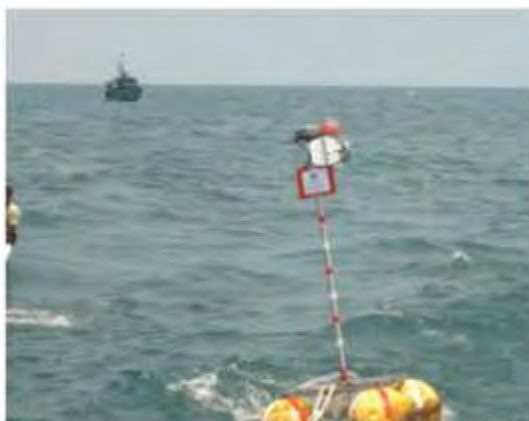
ANMS (with INSAT communication) deployment off Chennai during March 2016
