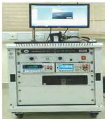
Calibration setup of Data Acquisition System
