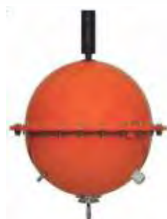
SST mounted in drifting buoy (Pradyu)
