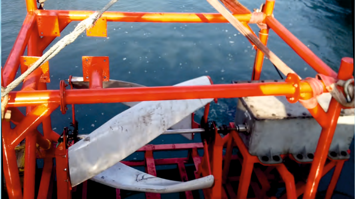
0.8 m diameter straight bladed vertical axis cross flow ocean current turbine being tested at open channel
