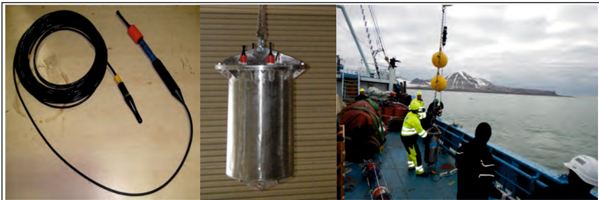
Hydrophone and DAQ with Underwater Pressure casing
