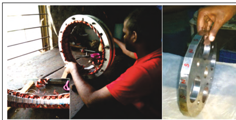
Stator coil assembly and rotor for 1 kW, 250 rpm PMSG
