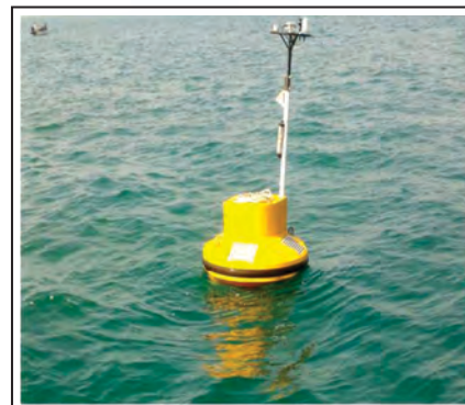
Coastal buoy with GPRS telemetry
