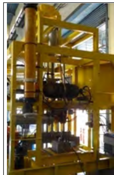
In-situ soil tester with vibration sinkage system
