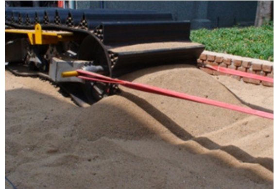
Undercarriage testing on sandy terrain
