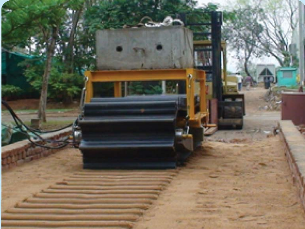
Undercarriage testing on sandy terrain
