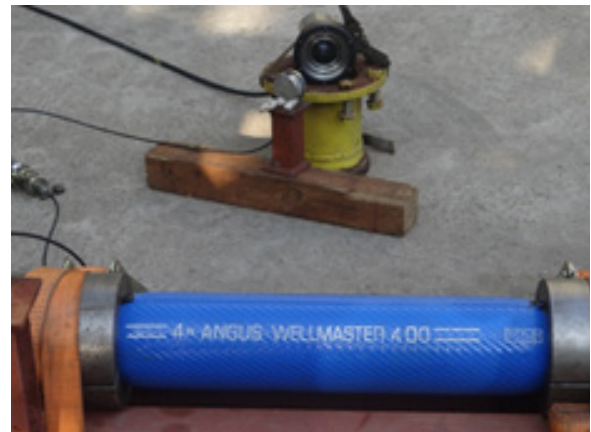
Hose testing for maximum burst pressure
