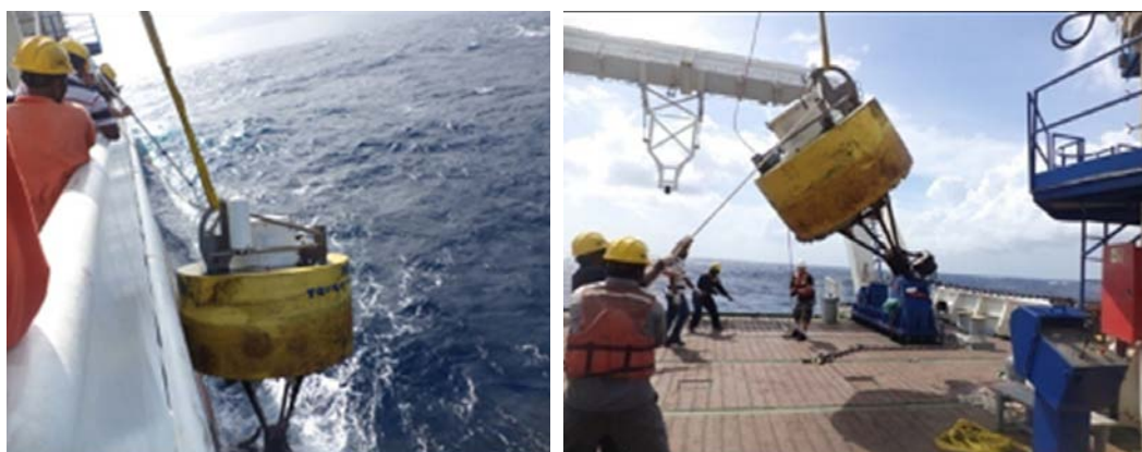
Deployment and retrieval of SAIC-INCOIS buoys
