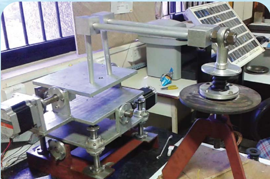
Studies on Interface system for the proposed 10 MLD offshore desalination plant with motion simulator built In-house
