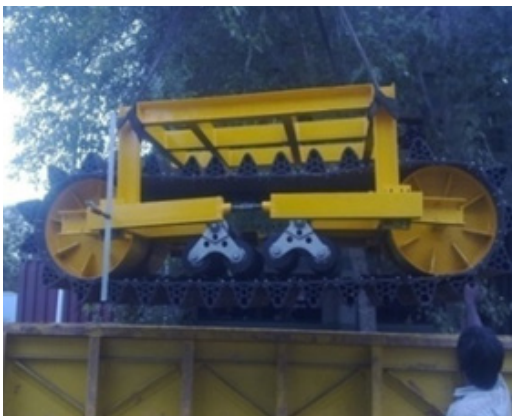
Undercarriage sinkage and pullout tests
