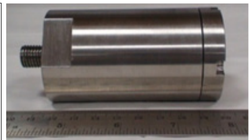
Indigenously developed Underwater Accelerometer for 6000 m depth
