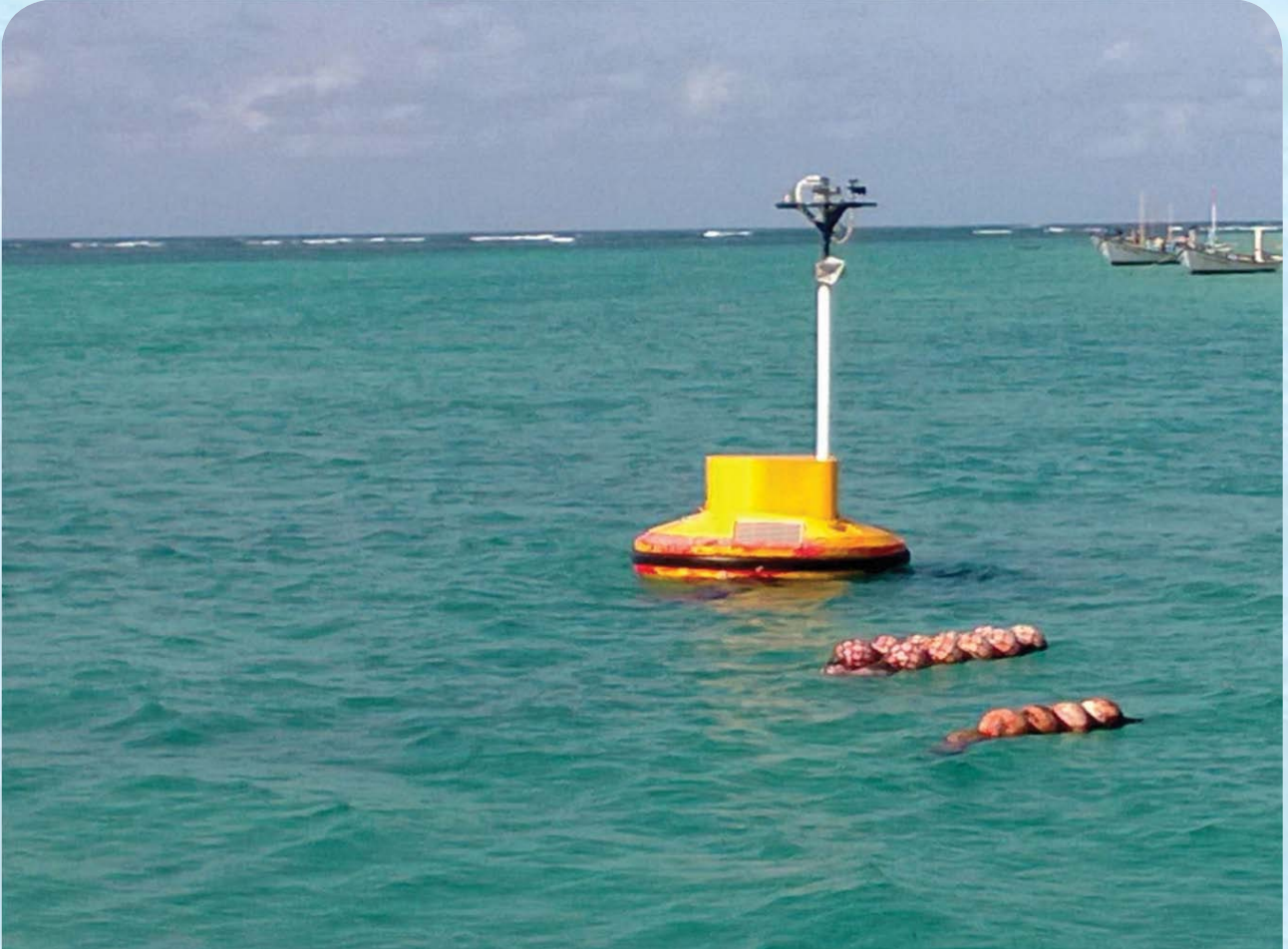
Coastal buoy system interfaced with INSAT and GPRS communication
