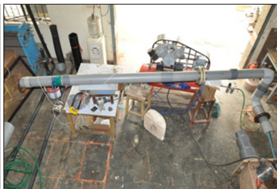
Orifice calibration setup using compressed air built at ESSO-NIOT
