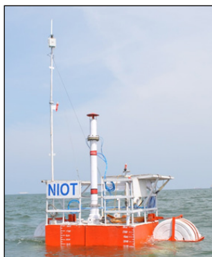
Backward bent ducted buoy equipped with calibrated orifices and air flow meter deployed at Kamarajar Port
