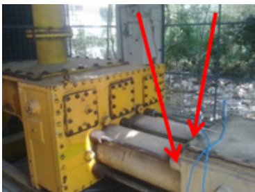
Accelerometers mounted on slurry Pump during operations
