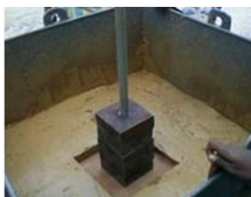
Soft feet ground bearing strength test setup
