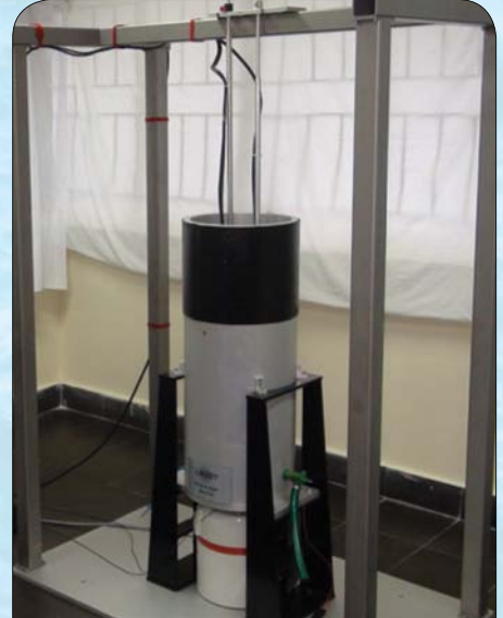
Low frequency calibration setup at Acoustic Test Facility
