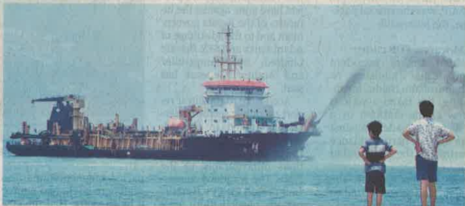
Mechanical wonder: A hi-tech dredger of the Dredging Corporation of India pumping sand using the rainbow technique at the old pier in Puducherry on Tuesday. ■ T. SINGARAVELOU
