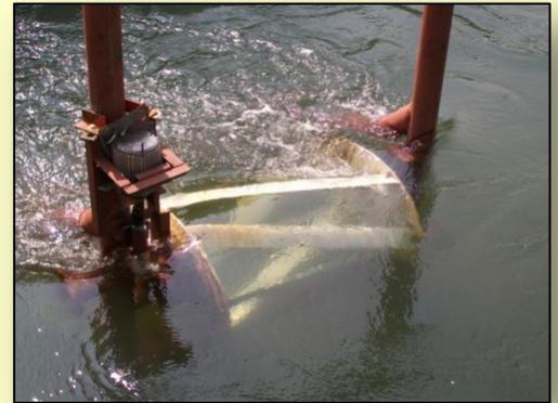
Testing of Inclined current turbine
